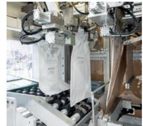
The fully automatic System-T FFS bagging machine combines high-quality packaging in a tubular PE bag with a high production capacity. This makes it ideal to be used in several fields, including the petrochemical, fertilizer, animal feed and food industries.
